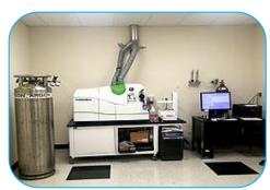
components, such as Na, K, Ca, Mg, can give serious damage lo mass spectrometer and the disposition of matrix constituents on the sampler and skinner cones of the Spectrometer, which can seriously affect the accuracy analytical results. Therefore, the matrices must be removed from the sample solutions before measurement by ICP-MS. In addition the preconcentration procedure is necessary when heavy metals exist at extremely low level to achieve more accurate measurement.
