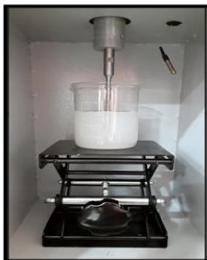
Figure no. 7:- Beaker contains dispersed ZnO, TiO 2 nanoparticles solution and plain white cotton fabric for coating
