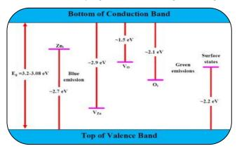
Al-ZnO thin film, electrons contributing from oxygen ions showed an increase in  $PO_2$ . The photoluminescence (PL) spectra of the films show the emission peaks visible from the faulty state. The optical properties of thin films confirm their applicability to optoelectronic devices. Room temperature, current-voltage (I-V) plot shows low resistivity in thin films ~ 10-2 ( $\Omega$ -cm).
