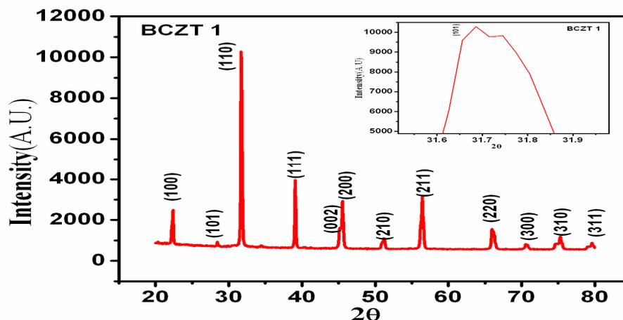
Figure 1: XRD pattern of BCZT1 ceramic.
