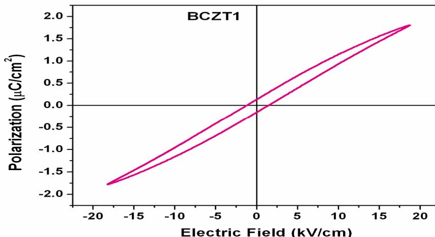
Figure 3: Ferroelectric hysteresis Loop of BCZT1 composition
