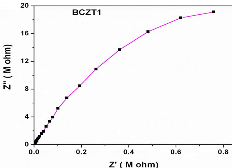
Figure 4:  $Z''$  Vs.  $Z'$  for BCZT1 composition.
